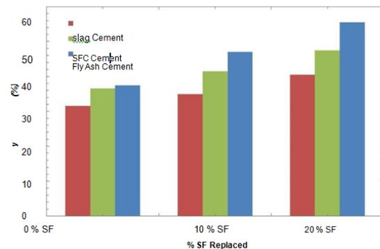
Figure.4.1.Consistency of Mortar.
