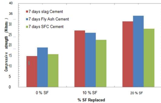
Figure.4.2 Compressive strength for mortar for 7 days
