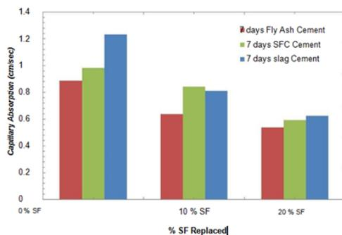
Figure.4.4 Capillary Absorption for mortar for 7 days
