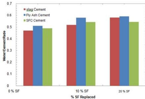
Figure.4.8 Water Cement Ratio for steel slag concrete
