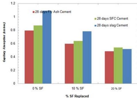
Figure.4.5 Capillary Absorption for mortar for 28 days
