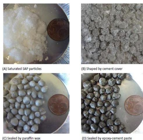
Figure 4.2 Manufacture of the capsules
