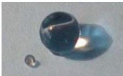
Figure 2.4 Dry, collapsed and a swollen suspension polymerized SAP particle [10]
