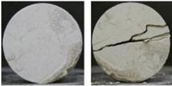
Fig: Split Tensile strength of concrete
