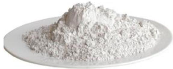
**Ground Granulated Blast Furnace Slag (GGBFS)**
