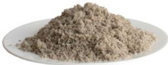
**Granulated Blast Furnace Slag**
