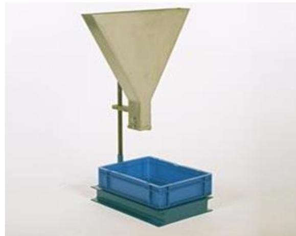
Fig: V-Funnel Test And Funnel Test At T5 Minutes
