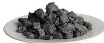
**Blast Furnace Rock Slag**
