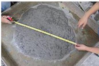
Fig 5.1: flow Slump dimensions
