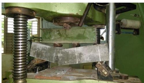
Fig- 5.4 Flexural testing machine with specimen
