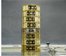
Fig - 4.3 sieve analysis apparatus
