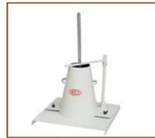
Fig - 4.1 slump test apparatus
