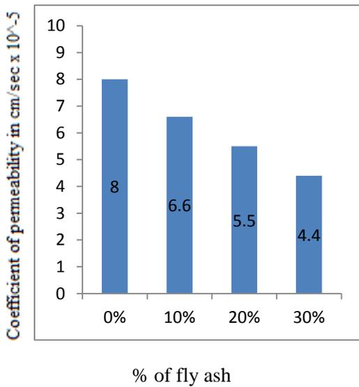
Fig: Relationship between % of fly ash and coefficient of permeability M20 grade concrete (RAC)
