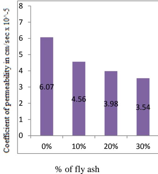
Fig: Relationship between % of fly ash and coefficient of permeability M35 grade concrete (RAC)
