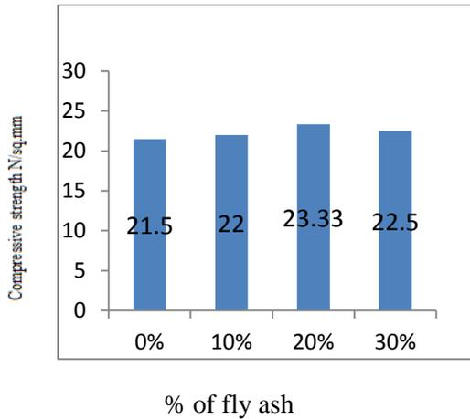
Fig: Relationship between % of fly ash and compressive strength of M20 grade concrete (RAC)
