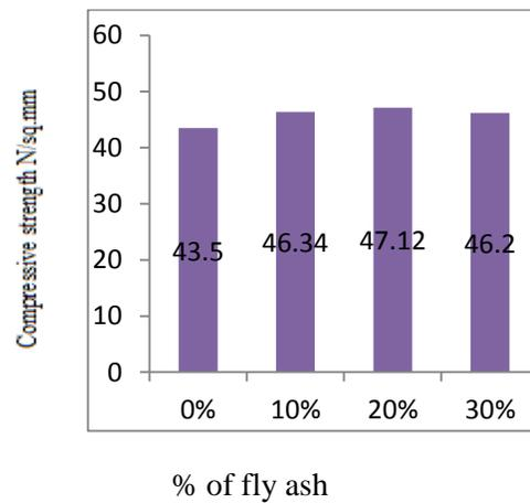
Fig: Relationship between % of fly ash and compressive strength of M35 grade concrete (RAC)
