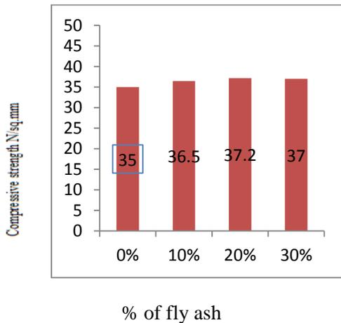
Fig: Relationship between % of fly ash and compressive strength of M25 grade concrete (RAC)
