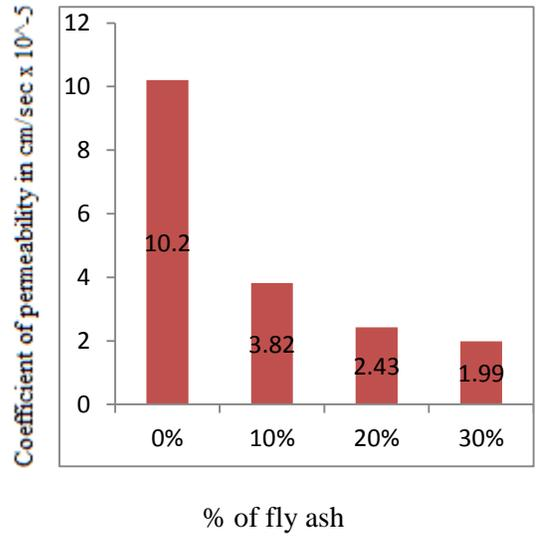
Fig: Relationship between % of fly ash and coefficient of permeability M25 grade concrete (RAC)
