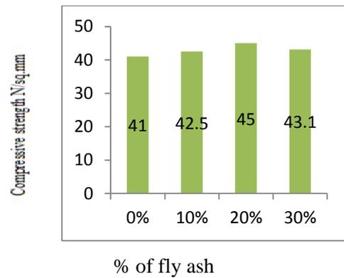
Fig: Relationship between % of fly ash and compressive strength of M30 grade concrete (RAC)
