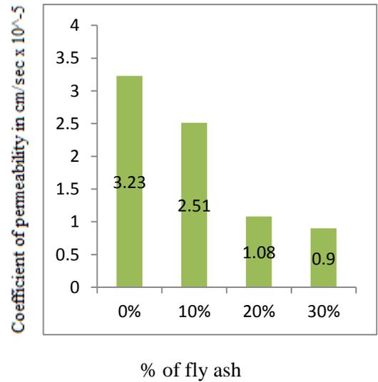
Fig: Relationship between % of fly ash and coefficient of permeability M30 grade concrete (RAC)
