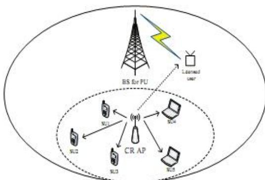
Fig.1. Cognitive Radio Architecture
