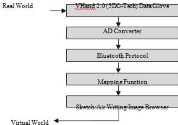
Figure 1. Hand Data Glove-Based Digital Sketching and Air-Writing System.
