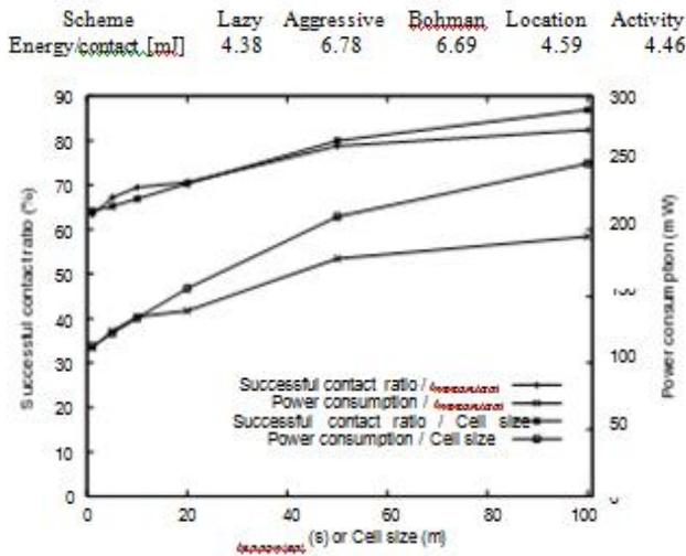
Fig.10. Performance of the adaptive recent-activity scheme versus time/contact and performance of the adaptive location-based scheme versus cell size
