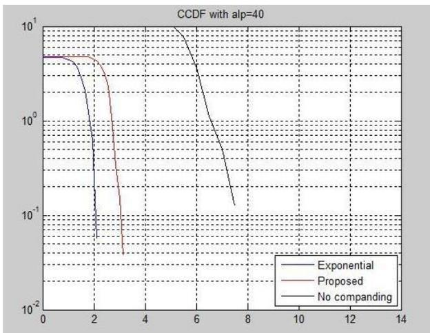
Fig:1. Complementary cumulative distribution function of original and companded signals (compander input power =30dBm,  $\alpha=40$ )
