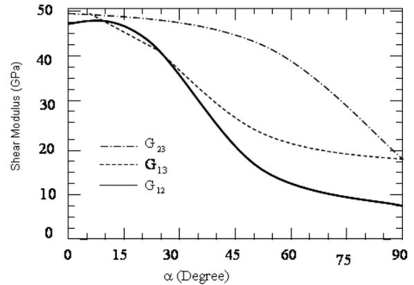
Fig.6. The effect of debonding angle on the composite shear moduli for doubly-symmetric debonding.
