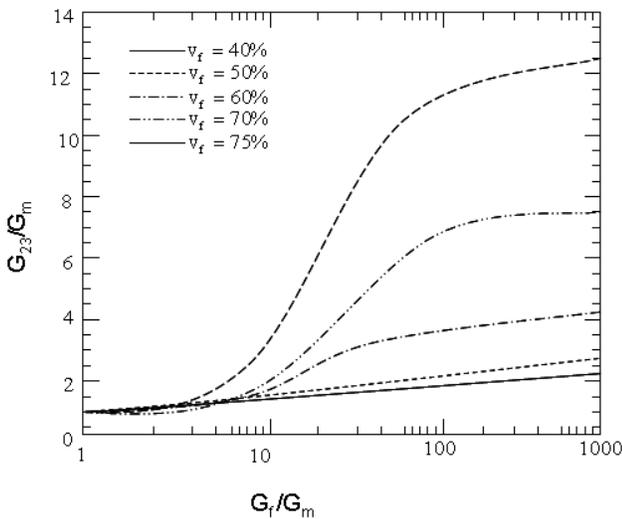
Fig.8. Effect of fiber volume fraction on the composite shear moduli  $G_{23}$  for perfectly bonded interface.
