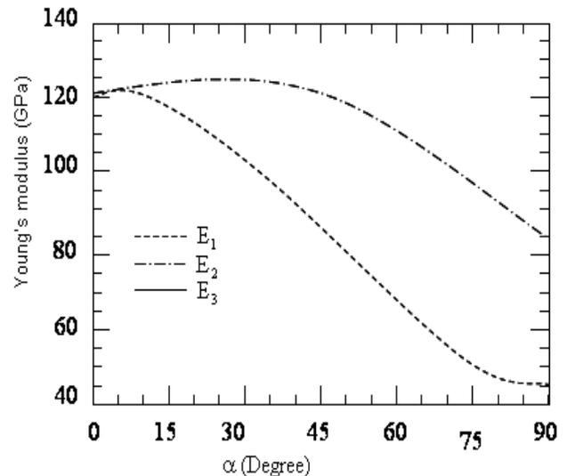
Fig.2. The effect of debonding angle on the composite Young's moduli for uni-symmetric debonding.
