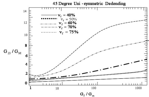
Fig.10. Effect of fiber volume fraction on the composite shear moduli  $G_{23}$  for uni-symmetrically  $45^\circ$  bonded interface.
