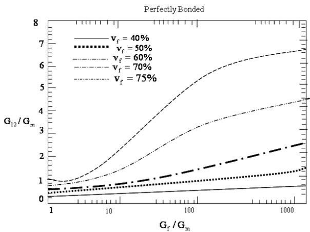
Fig.9. Effect of fiber volume fraction on the composite shear moduli for perfectly bonded interface. 12 G
