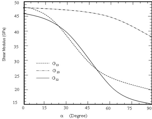
Fig.3. The effect of debonding angle on the composite shear moduli for uni-symmetric debonding.
