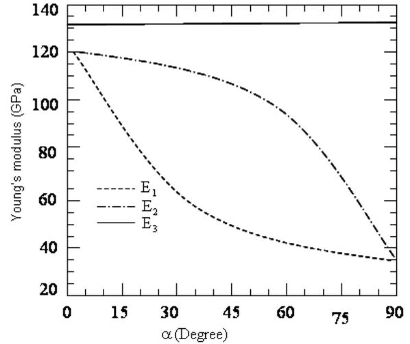
Fig.5. The effect of debonding angle on the composite Young's moduli for doubly-symmetric debonding.
