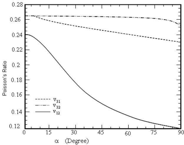
Fig.4. The effect of debonding angle on the composite Poisson's ratio for uni-symmetric debonding.
