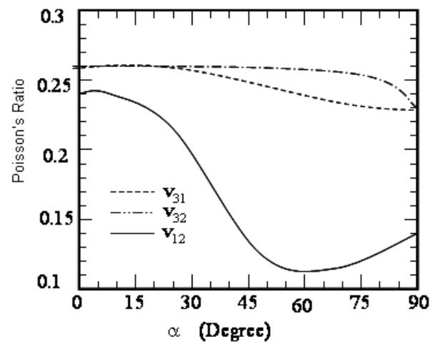
Fig.7. The effect of debonding angle on the composite Poisson's ratio for doubly-symmetric debonding.
