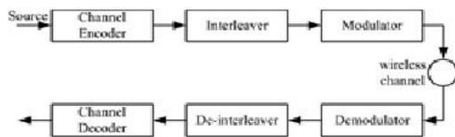
Fig.2. A generic communication system diagram.
